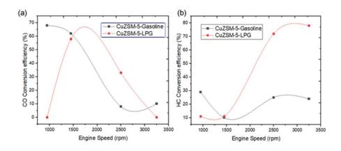
Figure 4: (a) CO reduction as a function of speed and (b) HC reduction as a function of speed
