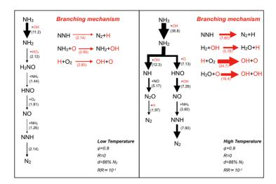
Figure 3. Flux diagram at R=0 and *φ*=0.9 for LT and HT regimes.
