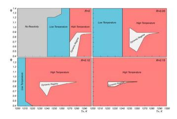
Figure 2. Numerical maps of combustion behaviors for NH<sub>3</sub>-H<sub>2</sub>/O<sub>2</sub>/N<sub>2</sub> mixtures for R=0, 0.05, 0.10, 0.15, diluted at 86% in N<sub>2</sub>, at p=1.2 atm and  $\tau$ =0.21 s.
