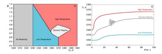
Figure 1. Experimental Map of combustion behaviors and characteristic  $T_r$  profiles for NH<sub>3</sub>/O<sub>2</sub>/N<sub>2</sub> mixtures diluted at 86% in N<sub>2</sub>, at p=1.2 atm and  $\tau$ =0.21 s.
