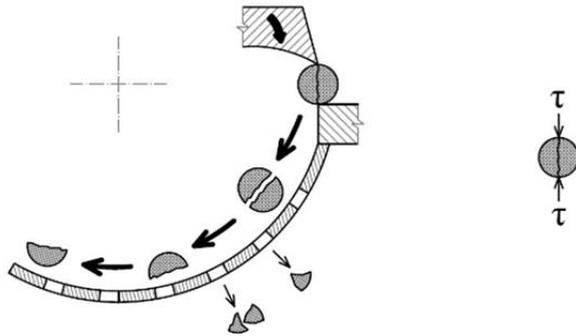
Figure 1: Basic principle of knife mill operation and particle shear stress
