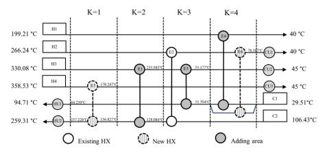
Figure 3: Optimal retrofitting HEN configuration by GAMS.
