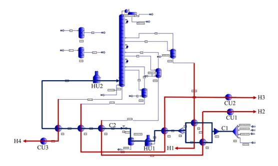
Figure 4: Process flow diagram of retrofitted crude preheat train validated by PRO II.
