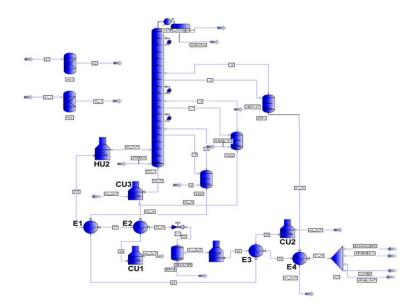
Figure 2: Existing process flow diagram for base-case crude preheat train by PRO/II
