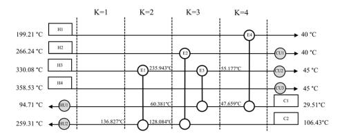
Figure 1 Existing grid diagram for base-case crude preheat train
