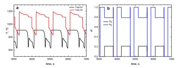
Figure 2: Outlet gas temperature (a) and N<sub>2</sub>-O<sub>2</sub> concentrations (b) vs time for first and second OC.
