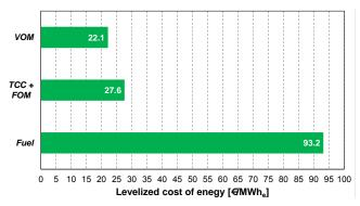
Figure 4: Levelized cost of energy for the TS-CLC, split in the three main contributions
