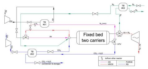
Figure 3: Sketch of the reactor network for the TS-CLC. HTV = high temperature valve, TB = thermal buffer
