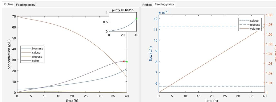
Figure 2. Process evolution with a constant feed flow of sugars for the likely most economic process ( $t_f = 40$  h,  $f = 0.14$ , total glucose added = 9.89 g).
