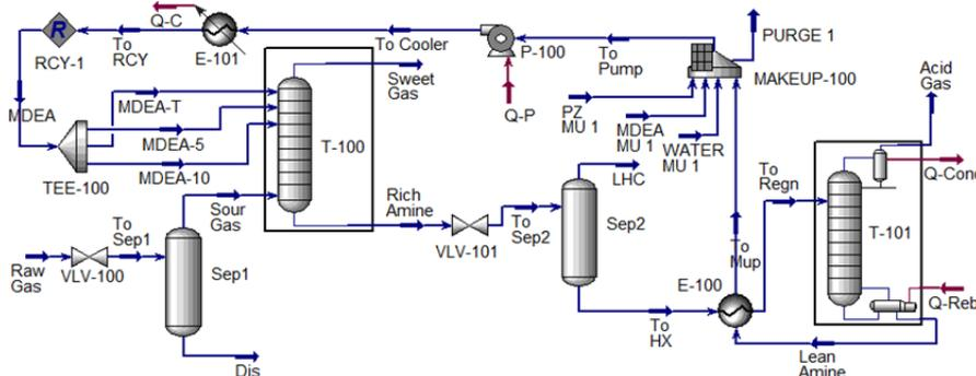
Figure 4: Process flow diagram for Sahel sweetening unit by Aspen HYSYS software.
