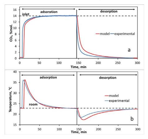
Figure 1: Comparison of modelled (red) and experimental (blue) breakthrough profiles over time for an inlet  $CO_2$  concentration (dashed black line) set at 14 mol.%. Vertical black line at 143 min indicates the switch between adsorption and desorption. To best fit the experimental data, the model assumes an initial  $CO_2$  fugacity in the bed of 3 mbar and an external heat transfer coefficient of 9 W/( $m^2 K$ ) (Boscherini et al., 2021)
