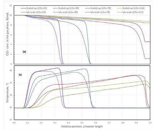
Figure 2: Simulated adsorption profiles in the sorbent bed of (a)  $CO_2$  gas concentration; and (b) temperature (b), plotted as function of dimensionless axial coordinate and dimensionless time (10%  $CO_2$  feed concentration): comparison between lab-scale (dashed lines) and scaled-up (continuous line) sorbent bed.
