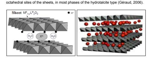
Figure 1: Schematic representation of a LDH phase structure (Géraud, 2006)
