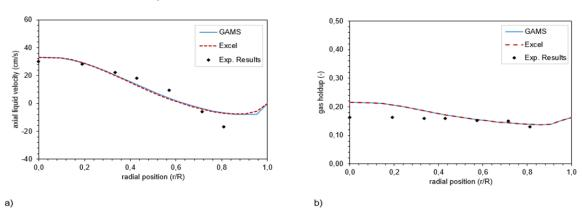
Figure 1- Results for (a) axial liquid velocity and (b) local gas holdup, comparing with experimental results from Yao et al. (1991).
