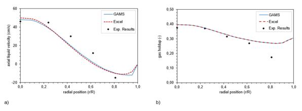
Figure 2- Results for (a) axial liquid velocity and (b) local gas holdup, comparing with experimental results from Torvik and Svendsen (1990).
