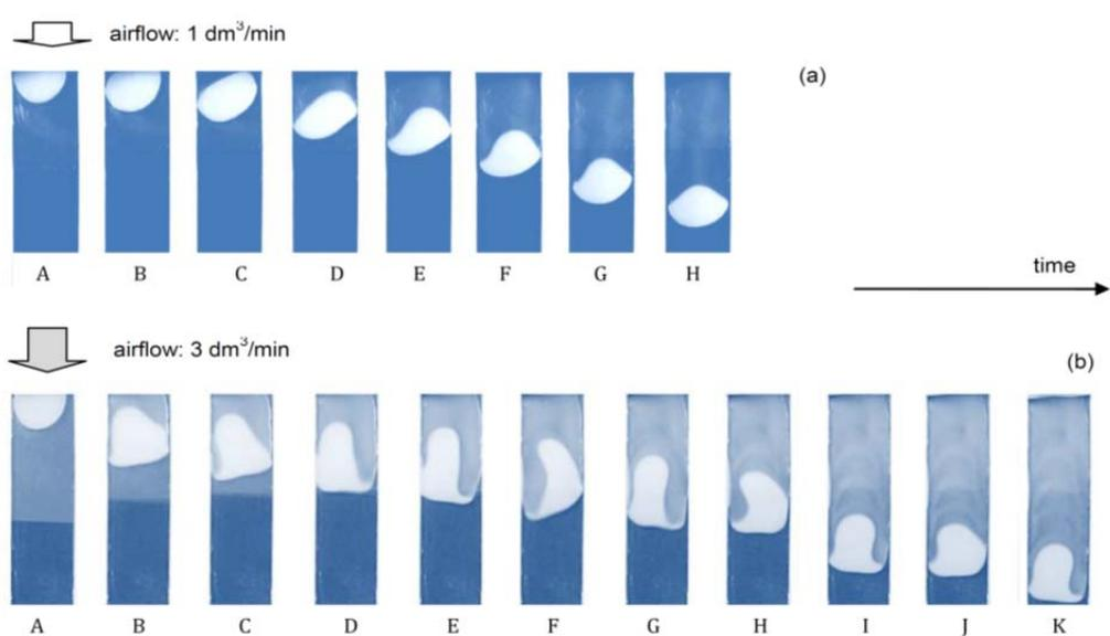
Figure 5: Displacement of a droplet of CMC+MIC 7.5% at two airflows: (a) 1 dm<sup>3</sup>/min, and (b) 3 dm<sup>3</sup>/min.
