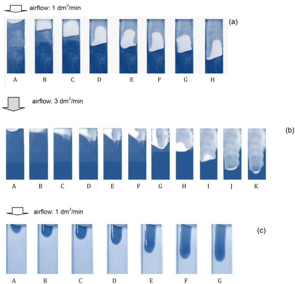
Figure 6: Displacement of a droplet: (a) CMC+MIC 7.5% on hydrophobic surface (airflow: 1 dm<sup>3</sup>/min); (b) CMC+MIC 12.5% (airflow: 3 dm<sup>3</sup>/min); (c) glycerol 70% aq. (airflow: 1 dm<sup>3</sup>/min).
