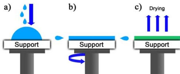
Figure 1: Scheme of spin-coating method used to prepare the nanocomposites: (a) few drops of toluene solution containing the BCP and NPs were deposited onto solid supports (glass or ITO-RCP supports); (b) the rotation at high spinning speed drove the solvent radically outward; (c) the complete evaporation of the solvent produced thin and uniform nanocomposite films; the morphology of the nanocomposite thin films was optimized by solvent or thermal annealing.
