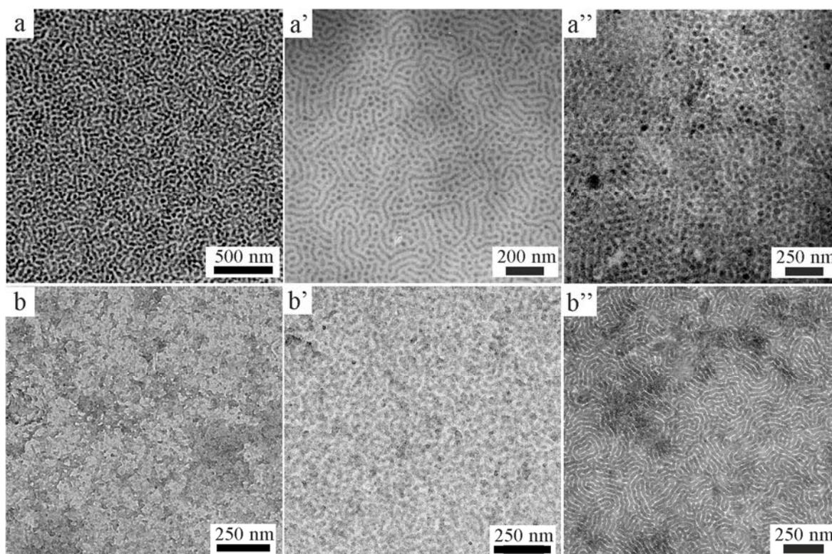
Figure 2: Bright-field TEM images of RuO<sub>4</sub>-stained thin films of neat BCPs prepared by spin-coating. Cyl-PSMMA thin films before (a) and after exposition to vapours of dichloromethane for 10 (a') and 20 (a'') min; Lam-PSMMA thin films before (b) and after thermal annealing at 190°C for 6 (b') and 24 (b'') hours.
