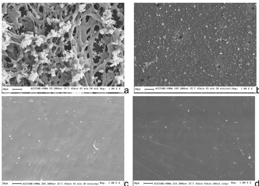
Figure 1. SEM images of PMMA surfaces obtained at 200 bar and 35°C, at different polymer concentration: a) 5% w/w, b) 10% w/w, c) 25% w/w, d) 50% w/w (scale bars = 20 µm).
