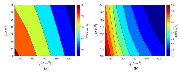
Figure 2: Contour maps of the Round Trip Efficiency a), and of the loss of Round Trip Efficiency due to parasitic currents b) as functions of the charge and discharge external current densities.
