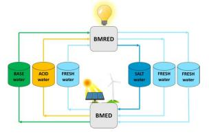
Figure 1: Acid/Base Flow Battery scheme (Culcasi et al., 2020a).
