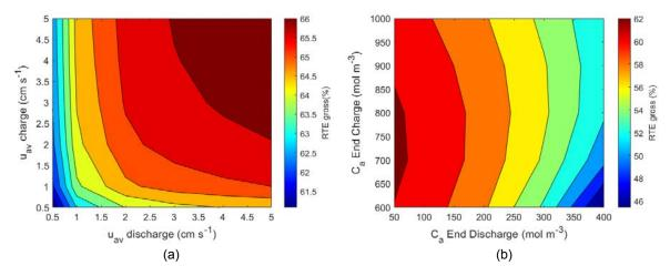
Figure 3: Contour maps of the Round Trip Efficiency as functions of a) the charge and discharge mean flow velocity and b) HCl concentration in the acid tank at the end of charge and discharge.
