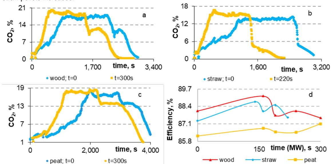
Figure 3: The effect of MW pretreatment time on the formation of  $\text{CO}_2$  emission for wood (a), straw (b) and peat (c) pellets and the average value of combustion efficiency (d).
