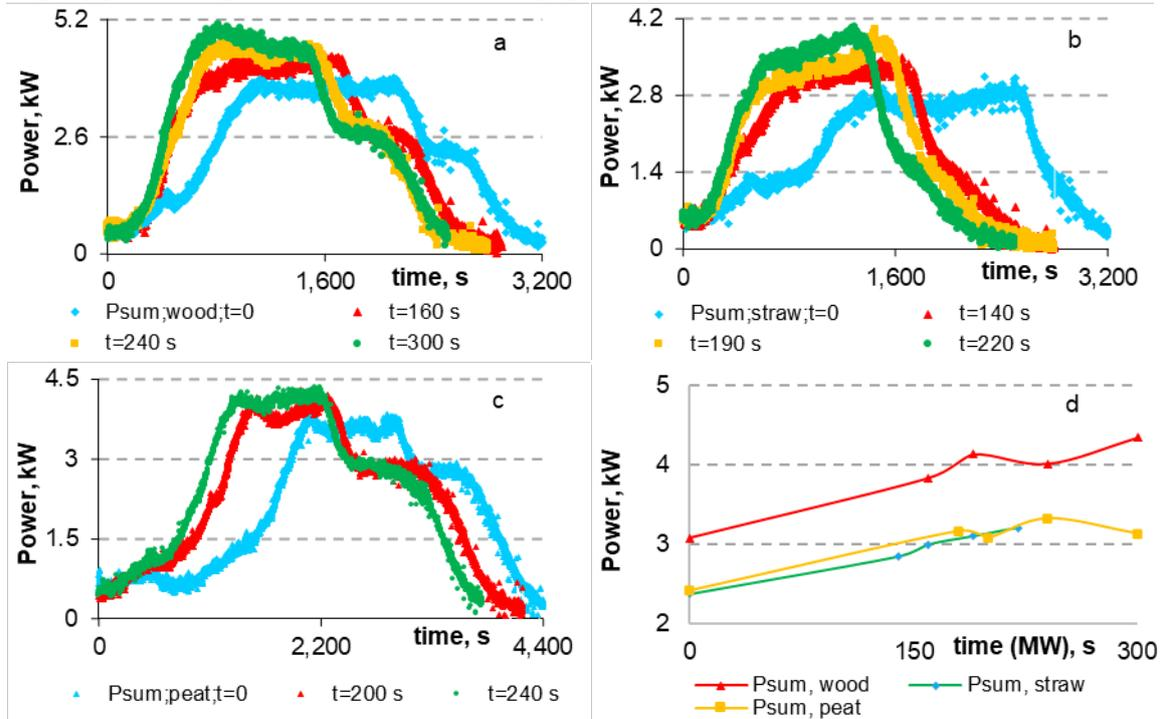
Figure 2: The effect of MW pre-treatment time of wood, straw, and peat pellets on kinetics of the heat output (a-c) and average values of the heat output from the setup in the flame reaction zone (d).
