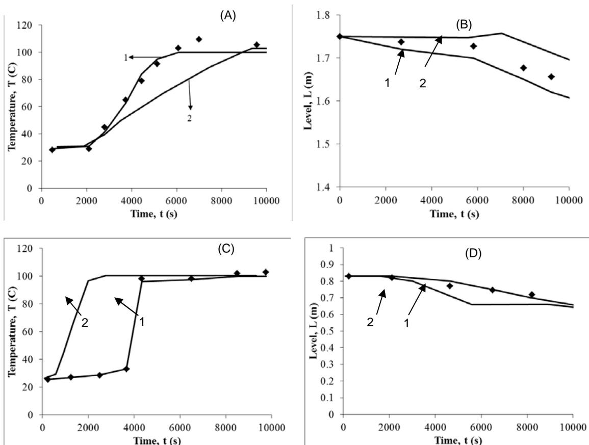
Figure 2: Comparison of model results with experimental data from literature. Temperature and level variation with time for (A), (B) Initial water level of 1.75 m. (C), (D) Initial water level of 0.83 m; ♦ Experimental data of literature (Sharma et al., 2008); 1. Present CFD Model 2. RELAP code
