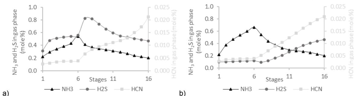
Figure 2: Concentration profile by the equilibrium-stage model (a) and rate-based model (b)
