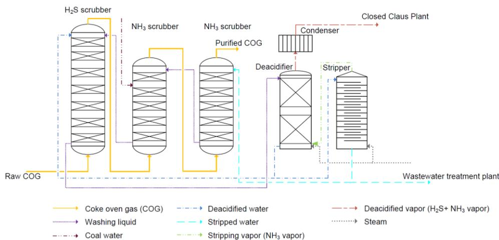
Figure 1: The coke oven gas purification technology
