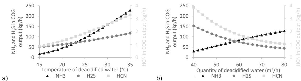
Figure 3: The effect of the temperature (a) and the quantity (b) of deacidified water on impurities in COG output flow
