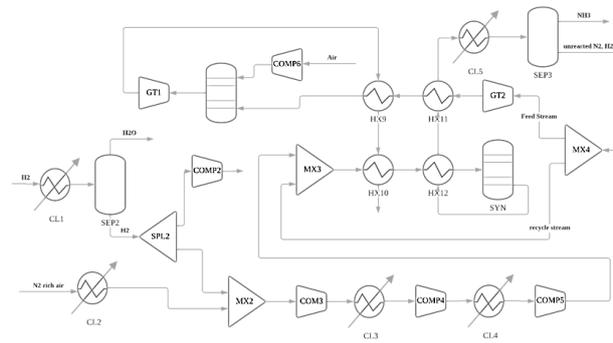
Figure 4: Process flow diagram of  $\text{NH}_3$  synthesis module.
