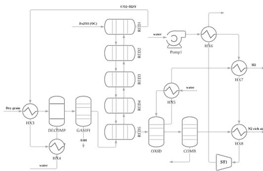
Figure 3: Process flow diagram of gasification, syngas chemical looping ( $\text{CLH}_2$ ).
