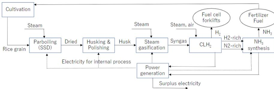
Figure 1: Schematic diagram of the proposed integrated system.
