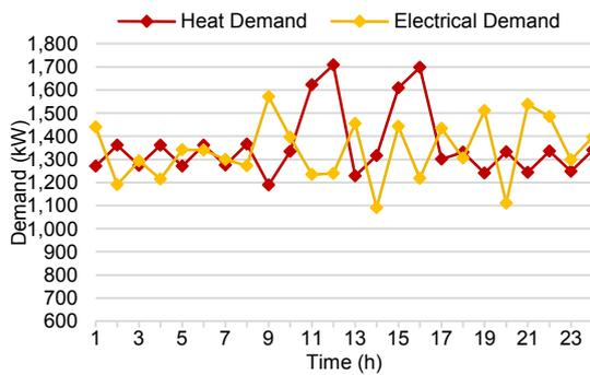
Figure 2: Energy demand loads of a pharmaceutical facility (adapted from Angizeh et al., 2020).
