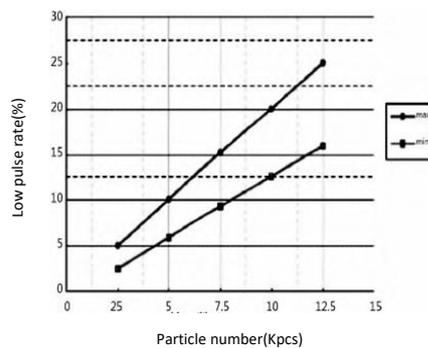
Figure 2: The relationship between the low pulse rate and the number of particles
