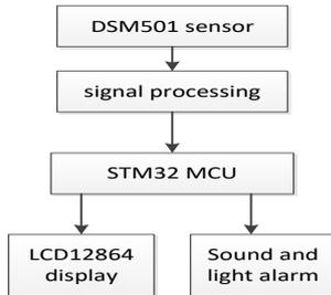
Figure 1: The principle block diagram of the PM2.5 detection system
