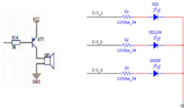
Figure 4: Sound and light alarm indicator circuit
