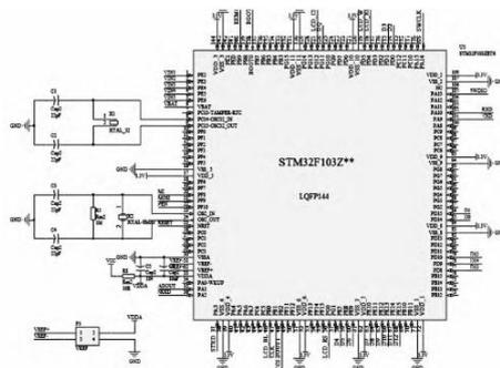
Figure 3: The smallest system of STM32
