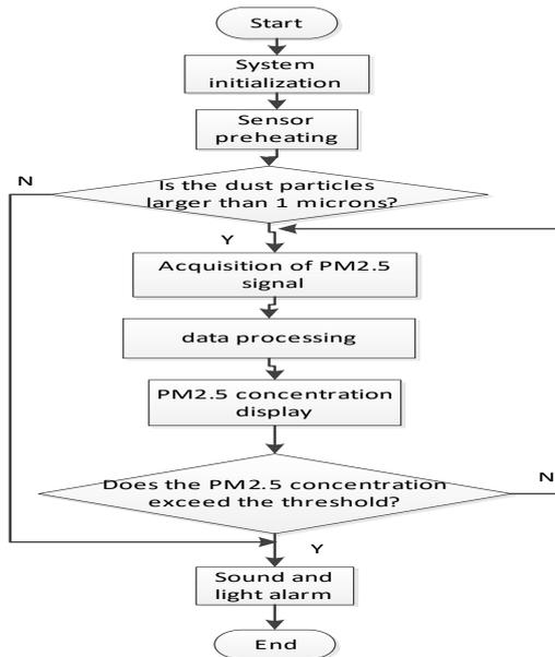
Figure 5: System software design flow
