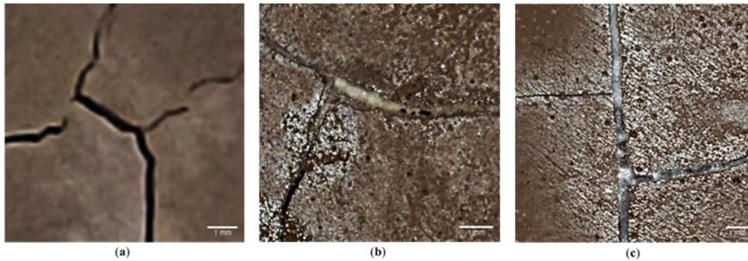
Figure 4: Crack sealing in a geopolymer after 28 healing days—(a) no healing agent; (b) using a pure culture of *B. sphaericus*, and (c) using co-culture of *B. sphaericus* and *B. thuringiensis*
