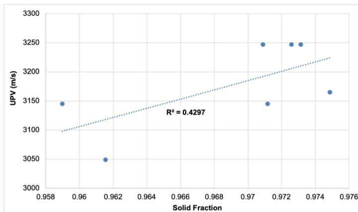
Figure 7: UPV versus the solid fraction of the geopolymers
