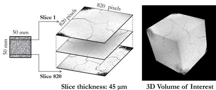
Figure 2: A reconstructed 3D image of a geopolymer cube from its VOI
