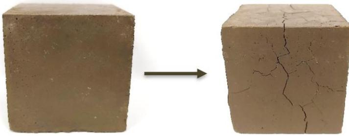
Figure 1: Thermally induced cracks in the geopolymers
