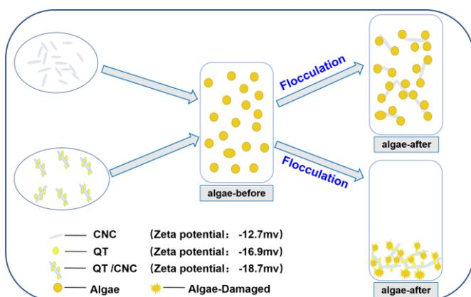
Figure 4: Schematic diagram for the Modification of QT/CNC and the removal of *Phaeocystis globosa*
