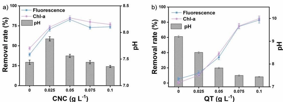
Figure 3: (a) Effect of CNC doses on algae removal. ([algal cell density] =  $1.5 \times 10^9$  cells  $L^{-1}$ , pH = 9.45,  $T = 25^\circ C$ , Time = 3h, [QT] =  $0.1 \text{ g } L^{-1}$ ) (b) Effect of QT doses on algae removal. ([algal cell density] =  $1.5 \times 10^9$  cells  $L^{-1}$ , pH = 9.45,  $T = 25^\circ C$ , Time = 3h, [CNC] =  $0.05 \text{ g } L^{-1}$ )
