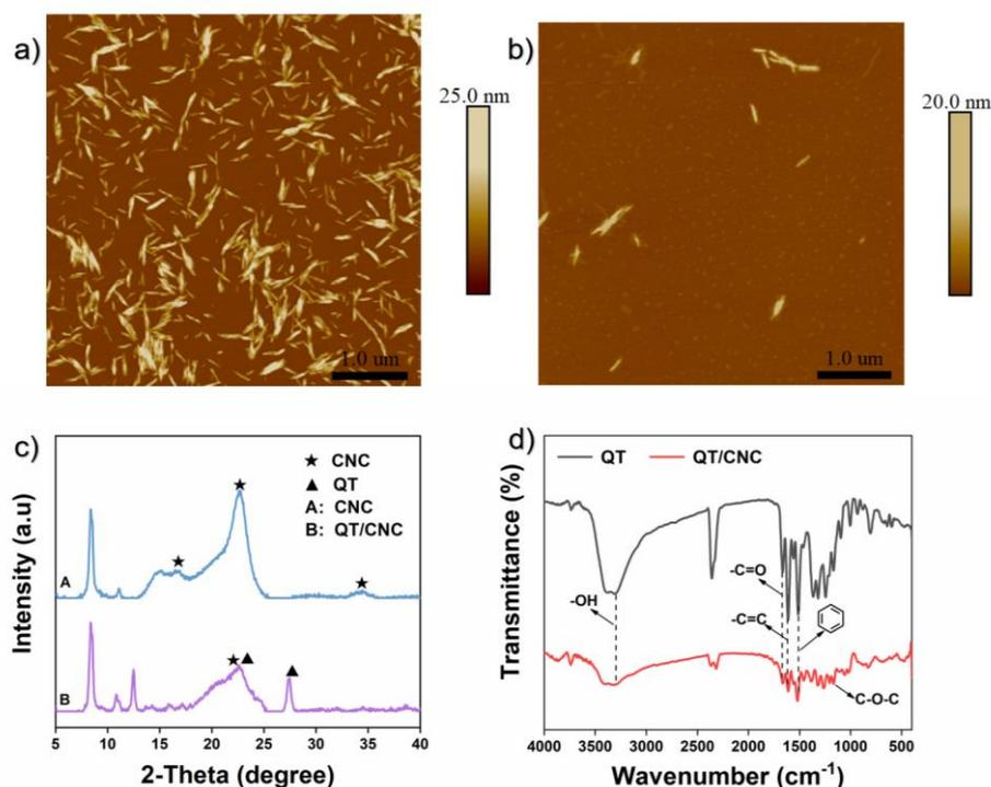
Figure 1: AFM height images of the (a) CNC and (b) QT/CNC; X-ray diffractograms of CNC and QT/CNC (c); FTIR spectra of QT and QT/CNC (d).
