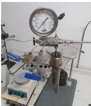
Figure 2: Experimental setup for hydrothermal decomposition of MER fibres in subcritical conditions
