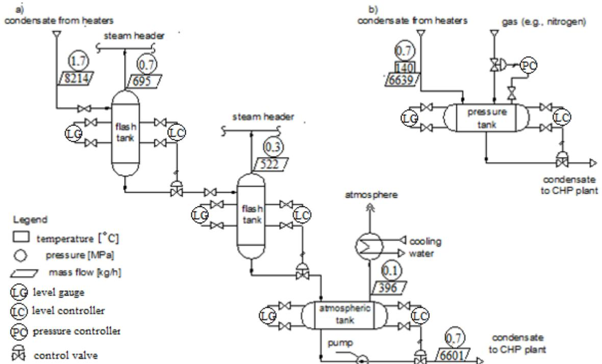
Figure 5: Scheme of condensate management in the MTBE plant: a) condensate flashing in the existing HEN arrangement, b) condensate tank connected to the retrofitted HEN
