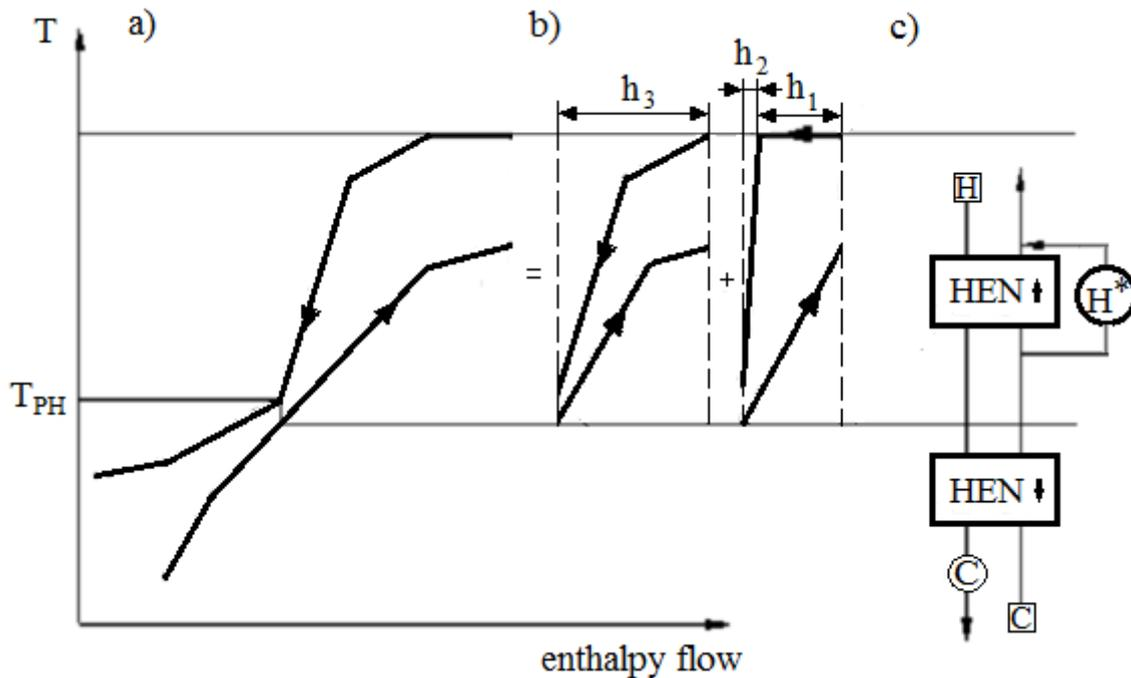
Figure 3: HEN retrofit concept to enable condensate subcooling in selected heaters denoted  $H^*$ : a) Balanced Composite Curves, b) temperature profiles of the heat exchange in heaters  $H^*$  [heat duty  $h_1$  and  $h_2$ ], and network part  $HEN^\dagger$  [heat duty  $h_3$ ], c) simplified block scheme of the HEN including its parts operated above and below Pinch temperature [ $HEN^\dagger$  and  $HEN^\ddagger$ ]; C – coolers
