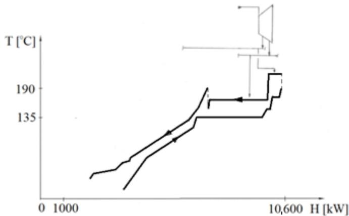
Figure 4: Balanced Composite Curves illustrating heat recovery with the subcooling of steam condensate, and symbolic representation of steam supplies from turbine extraction
