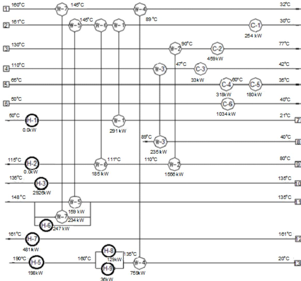
Figure 6: Grid diagram of the retrofitted HEN with the subcooling of steam condensate
