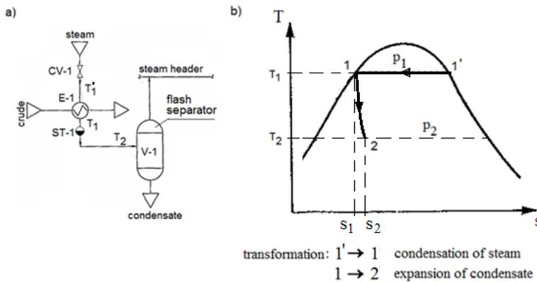
Figure 1: Heat supply from CHP plant to crude-oil heating: a) flow diagram; b) changes in the thermodynamic state of steam and its condensate in the T-s diagram
