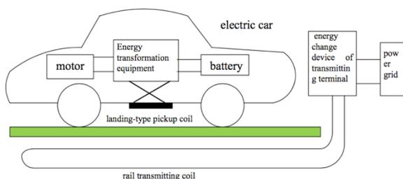
Figure 1: Wireless charging schematic diagram of landing-type scaffolding pick-up coil
