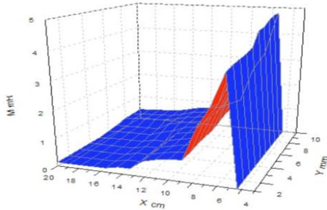
Figure 5: Variation curves of mutual inductance  $M$  changing along with primary and secondary side distance  $X$  and lateral motion  $Y$
