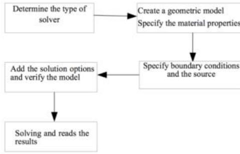
Figure 7: Steps and process to build a simulation model
