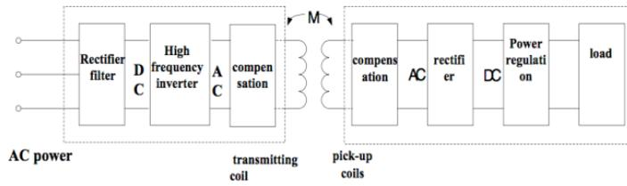
Figure 2: Power transmission system main circuit structure diagram
