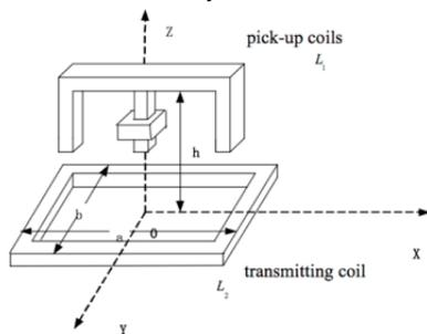
Figure 4: Schematic diagram of pickup coil and transmitter
