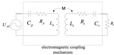
Figure 3: SS topology structure diagram
