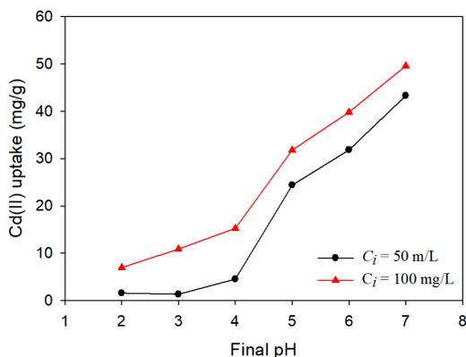
Figure 2: Effect of pH on Cd(II) uptake by PAA-PSBF
