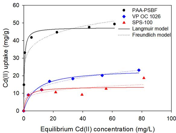
Figure 3: Adsorption isotherm of Cd(II) on PAA-PSBF, Lewatit® VP OC 1026, and SPS-100 at pH 7.
