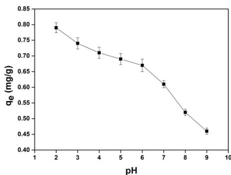
Figure 1: The effect of pH on Cr (VI) removal of FAZ adsorbent
