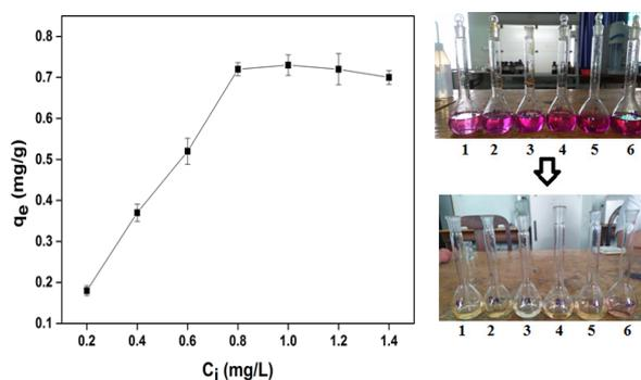
Figure 3: The effect initial Cr (VI) concentration on adsorption capacity
