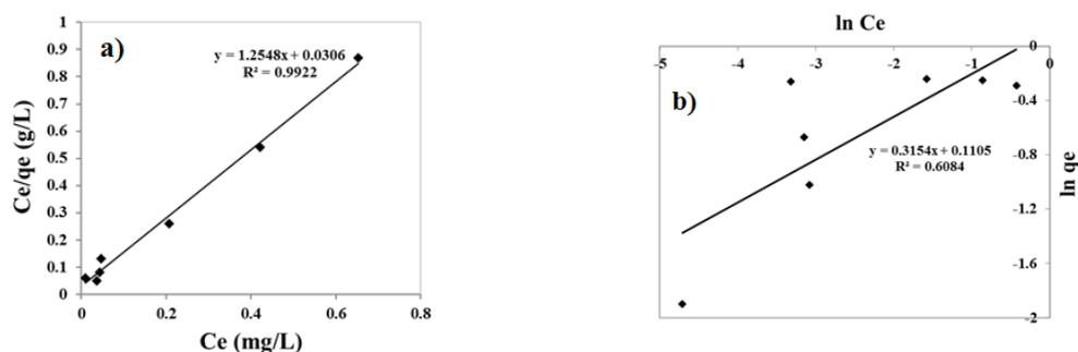
Figure 4: The isotherm schemes of Cr (VI) adsorption by FAZ: a) Langmuir model; b) Freundlich model
