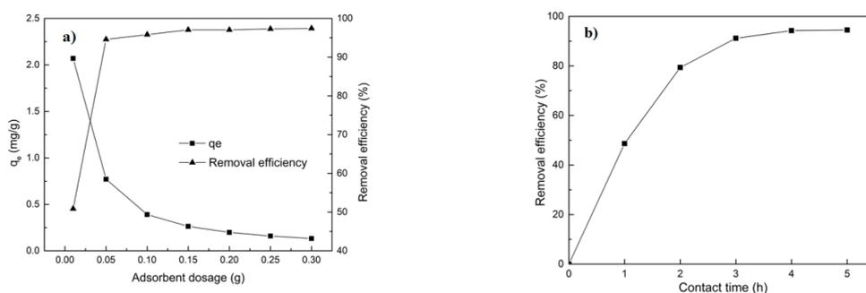
Figure 2: The effect adsorbent dosage (a) and contact time (b) on Cr (VI) adsorption
