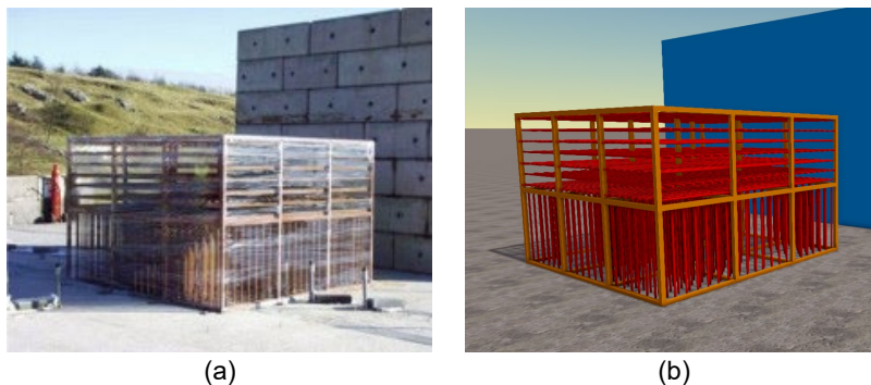
Figure 2: Experimental configuration (a) and geometry model in FLACS-CFD (b) for the 9-gate congestion type.
