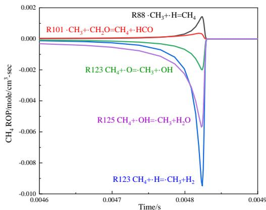
4c 9.5% CH<sub>4</sub>+4% H<sub>2</sub>
