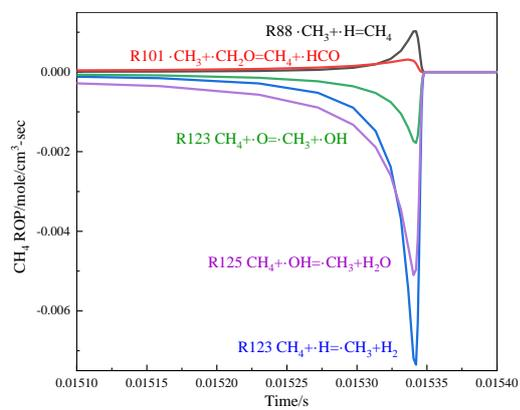
4d 9.5%CH<sub>4</sub>+0.2%C<sub>3</sub>H<sub>8</sub>+1%H<sub>2</sub>Figure 4: CH<sub>4</sub> ROP under different working conditions
