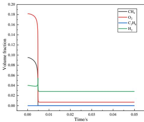
3c 9.5% CH<sub>4</sub>+4% H<sub>2</sub>
