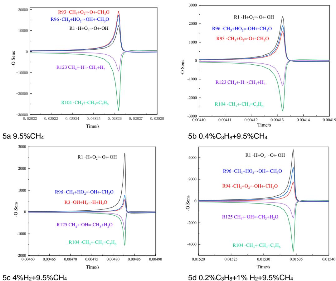
Figure 5: O sensitivities analysis under different working conditions
