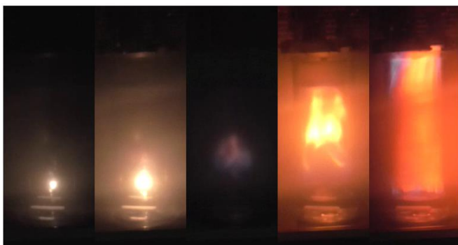
Figure 6: UEP: Flame development (left to right) in the gas phase (liquid temperature: 12.5°C) after spark generation
