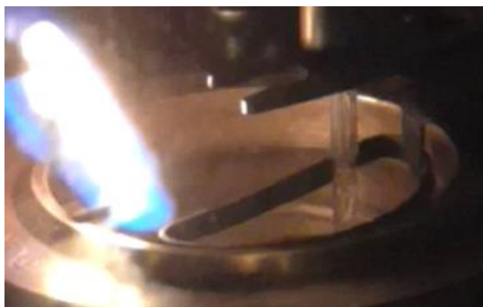
Figure 2: Pilot flame above the liquid ethoxy-nonafluorobutane at a temperature of 32°C (Open cup test performed at Ineris)
