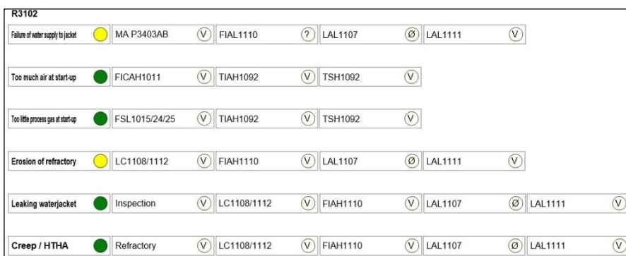
Figure 7: The process safety dashboard of the post reformer with multiple scenarios
