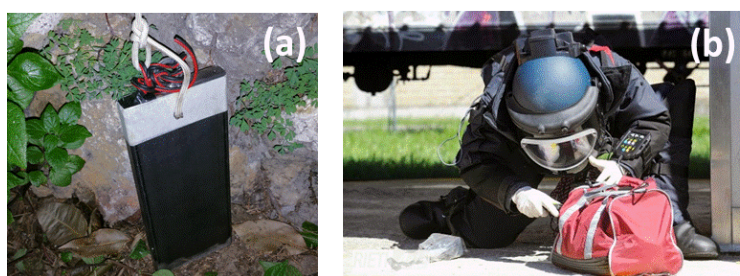
Figure 1: Panel (a): image of an IED, made of a metallic box containing a mixture of \text{NH}_4\text{NO}_3 and powdered Al, equipped with a homemade detonator, found in Liguria (Italy) and defused by one of the authors (F.C.). Panel (b): image of the same author dressing a safety equipment, during an inspection of a suspicious baggage.
