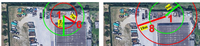
Figure 6: Safety distances (a) heap - paper bales and (b) heap - container.
