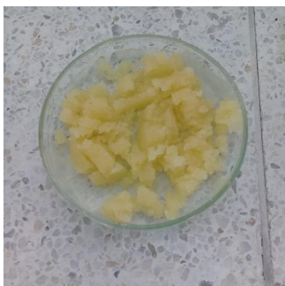
Figure 2: Biomass from cocoa husk pods after two alkali treatments.
