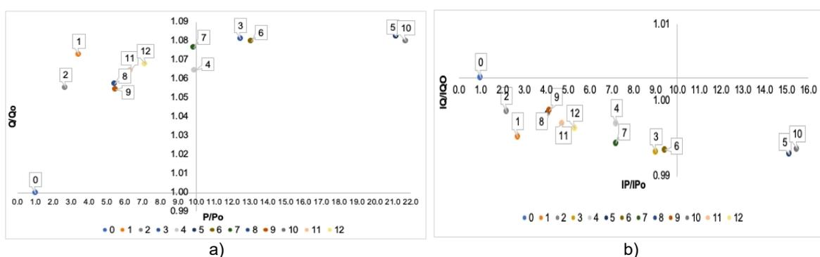
Figure 4: Turbulence promoter performance mapping for case study 1: a) Relative heat load vs relative pressure drop, b) Relative irreversibility due heat load vs relative irreversibility due to pressure drop.
