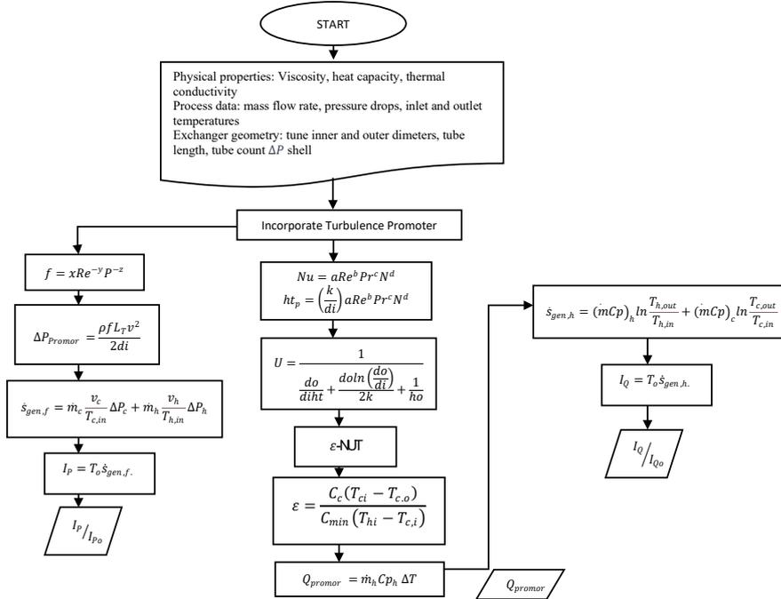
Figure 2: Flow chart of the computation of new thermal and pressure drop of a heat exchanger with turbulence promoters
