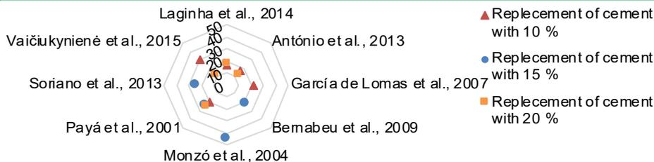
Figure 3: The impact of waste FCC catalyst on compressive strength enhancement of substituted composites
