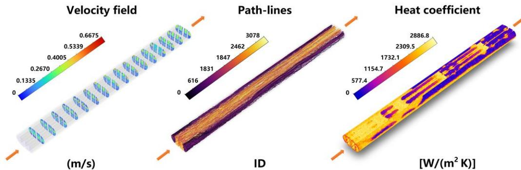
Figure 3: Flow heat transfer field contours including velocity, path lines, and heat coefficient
