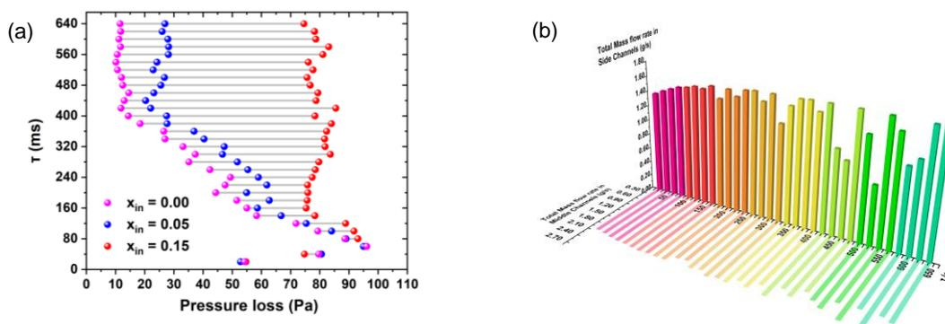
Figure 5: (a) Pressure drop between the inlet and outlet, (b) The total flow in the middle (M) and on both sides (S) of the elliptical tube microchannels
