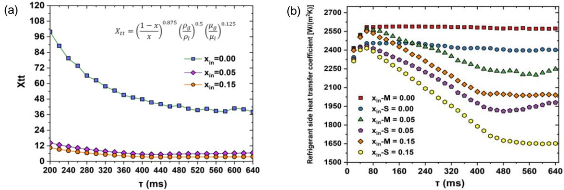
Figure 6: (a) Martinelli parameter ( $X_{tt}$ ) curve with boiling time, (b) The refrigerant side heat transfer coefficient
