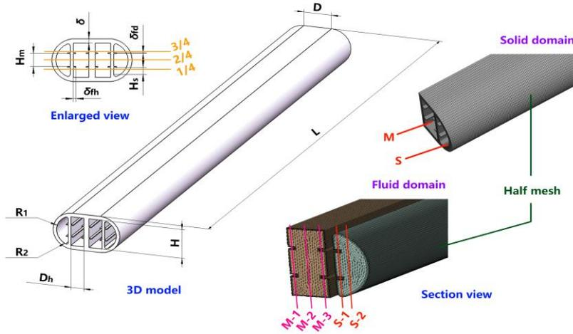
Figure 1: 3D model annotation and schematic and computational domain grids
