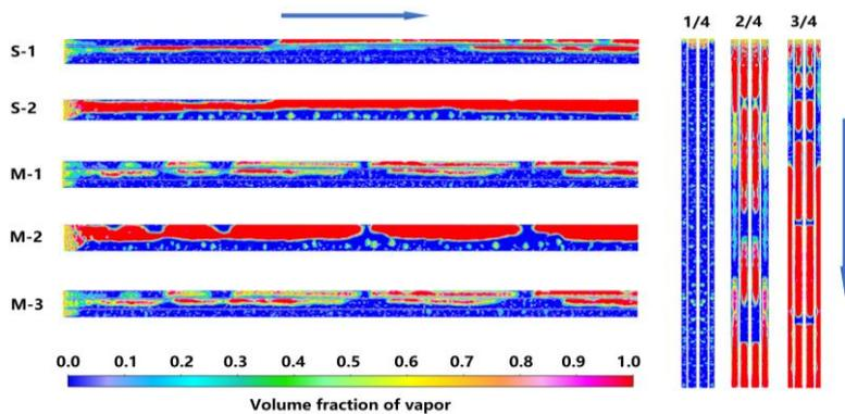
Figure 4: Flow pattern of gas-liquid two-phase flow during the boiling heat transfer process
