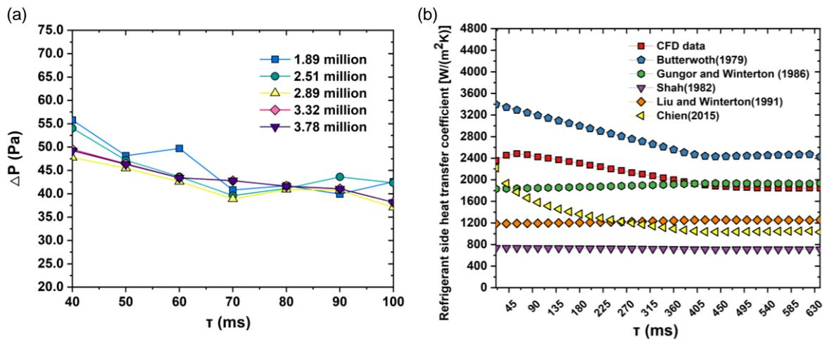
Figure 2: Methods validation: (a) Mesh independence validation, (b) Results validation
