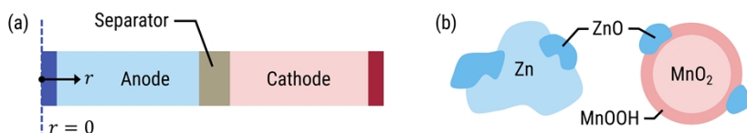
Figure 2: The battery is treated as a 1D axisymmetric system (a). The zinc anode is not modeled as any specific particle geometry, while the \text{MnO}_2 cathode is described via a core-shell model \text{MnOOH} (b).
