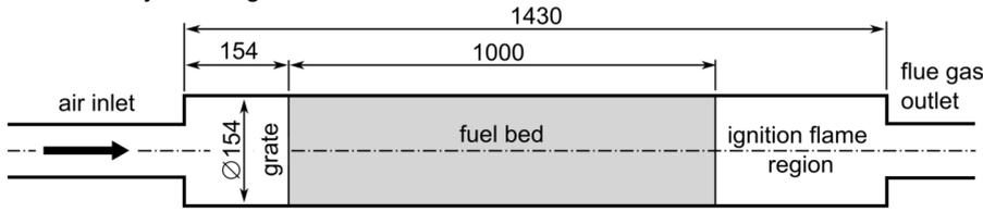
Figure 2: The model geometry, adapted from the description of the experimental reactor.
