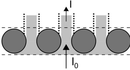
Figure 1: Particles' arrangement assumed by Shin and Choi (2000) for estimation of  $\beta_s$ . The grey area represents the actual transmitted radiation, dotted lines illustrate the amount of radiation as given by the proposed expression for  $\beta_s$ .
