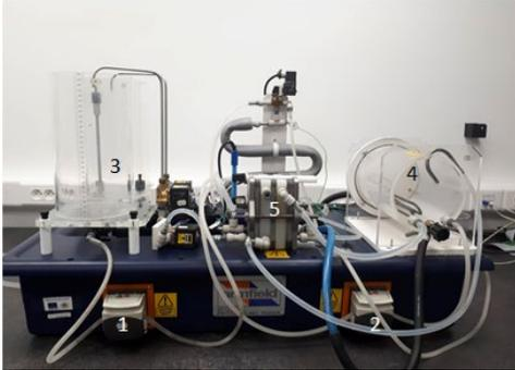
Figure 1: Laboratory heat exchanger Armfield Process Plant Trainer PCT23: cold medium (1) and heating medium (2) pumps, cold medium (3) and hot medium (4) tanks, heat exchanger (5)
