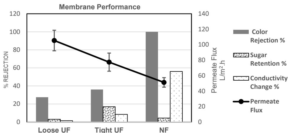
Figure 2: Performance of the membranes during filtration (Colour removal, Sugar permeability and Salt rejection) Operating parameters: 60 °C, 3.6 L/min, 8 bar for UF and 30 bar for NF. Permeate flux - Volume of permeate recollected during membrane separation per unit of time and membrane area.
