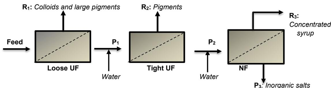
Figure 1: Diagram of decolourization of starch hydrolysates by an integrated membrane system ( $R$ =Retentate;  $P$ =Permeate).
