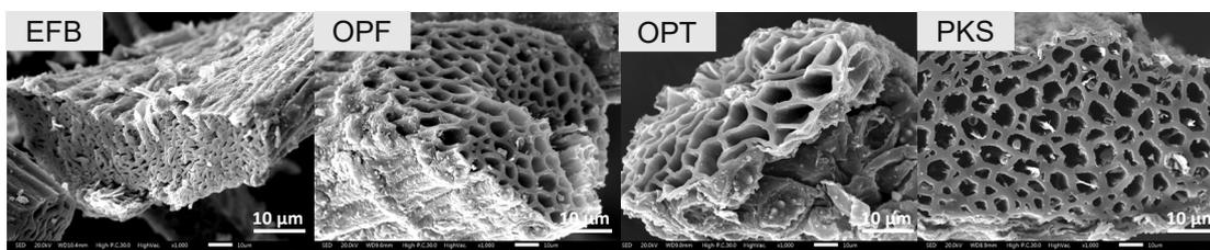
Figure 4: SEM images of biochar from pyrolysis of EFB, OPT, OPF and PKS (550 °C, 0.7 L/min, 75 min).
