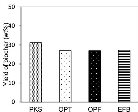
Figure 2: Biochar yield from various oil palm waste under optimum pyrolysis condition.
