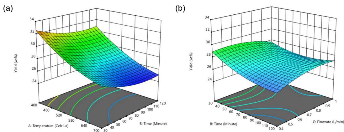
Figure 1: 3D response of: a) the effect of temperature ( $^{\circ}\text{C}$ ) and retention time (minutes), b) the effect of temperature ( $^{\circ}\text{C}$ ) and nitrogen flowrate (L/min) on the biochar yield.
