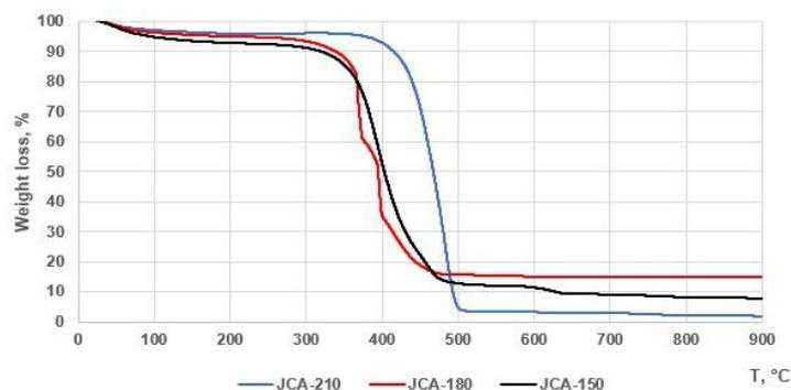
Figure 2: Thermogravimetric analysis (TGA) curves of different JCA samples
