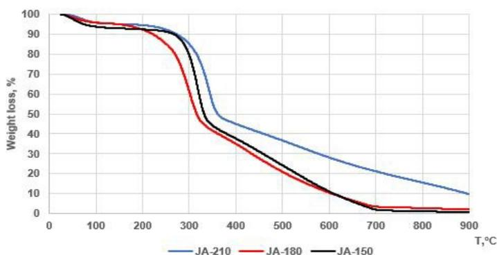
Figure 1: Thermogravimetric analysis (TGA) curves of different JA samples
