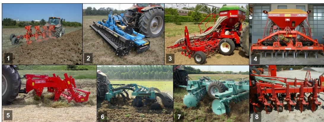
Figure 1: Tested implements. (1) four-furrow reversible plough, (2) rotary harrow, (3) pneumatic seed drill, (4) combined seeder, (5) subsoiler, (6) combined cultivator, (7) offset disk harrow, (8) pneumatic seed drill.
