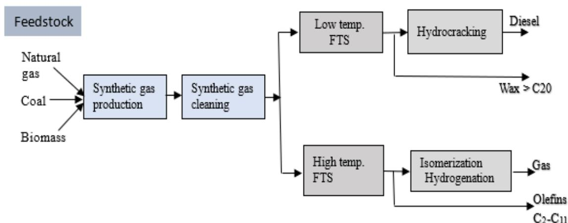
Figure 3: Fischer Tropsch Synthesis for green diesel production (Lff, 2015)
