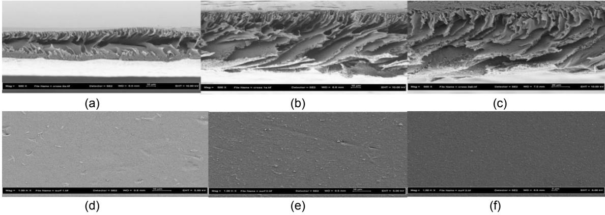
Figure 1: SEM micrographs of cross sections and surface of membranes at 1,000x magnification; Cross section (a) PES-HFO 0, (b) PES-HFO 0.5, (c) PES-HFO 1.0; Surface (d) PES-HFO 0, (e) PES-HFO 0.5, (f) PES-HFO 1.0
