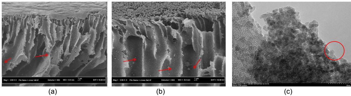
Figure 2: SEM micrographs of (a) PES-HFO 0.5, (b) PES-HFO 1.0, (c) TEM image of HFO
