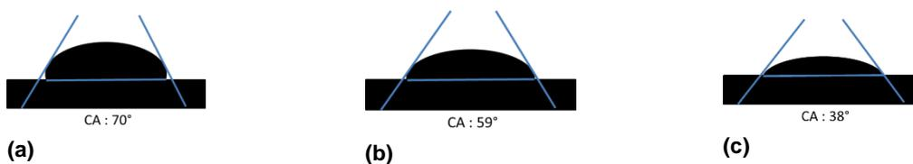
Figure 4: Water contact angle of membranes, (a) PES-HFO 0, (b) PES-HFO 0.5, (c) PES-HFO 1.0
