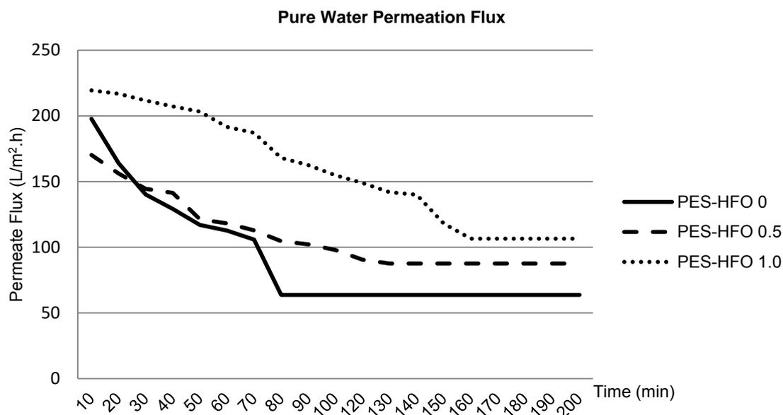
Figure 5: Pure water permeation flux of PES membrane with different loading of HFO
