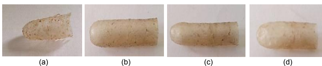
Figure 4: Photographs of hard seeds gum capsule shell from 3 %wt gum solution and varied proportion of plasticiser: (a) 0 %, (b) 2 %, (c) 5 %, and (d) 10 %
