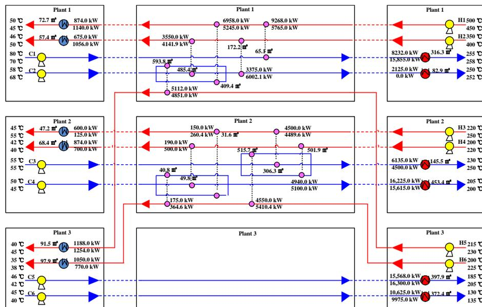
Figure 3: Heat exchanger networks for Multi-Plant Heat Integration.
