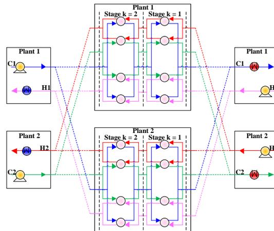
Figure 1: Superstructure for Multi-Plant Heat Integration considering multi-period operations
