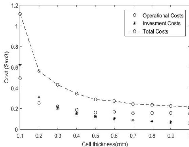
Figure 6. Cell thickness effect in the total cost of an ED systems for Pueblo Viejo, Colombia
