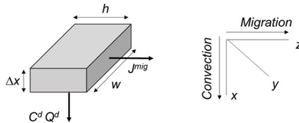
Figure 2. Differential volume to analyze the diluted flow across the ED system
