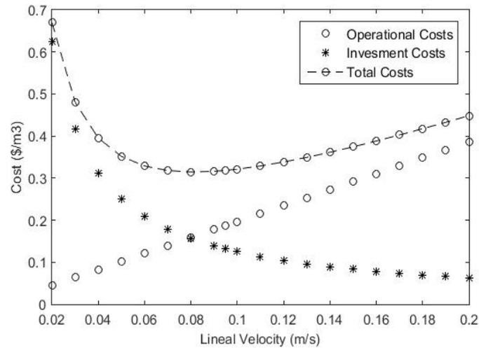
Figure 5. Linear velocity effect in the total cost of an ED systems for Pueblo Viejo, Colombia
