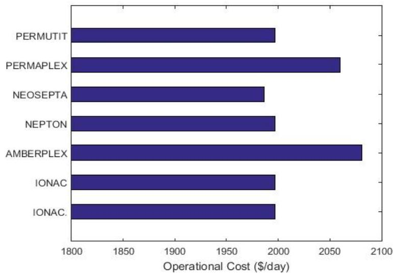
Figure 4. Cost comparison of operational costs using different types of membranes
