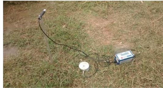
Figure 2: Monitoring of ground vibration with minimize plus seismograph
